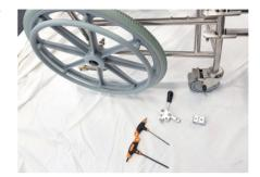
**2.** Install clamp between location pins at approx. 45° as shown in picture.
