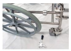
**3.** Install brake handle fixation rail into clamp.
