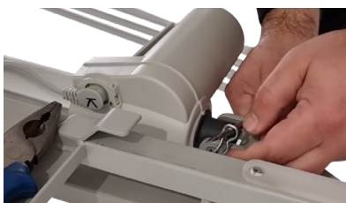
Step 11: Remove kneebreak actuator on opposite side. (Left hand side when lying on the bed)
