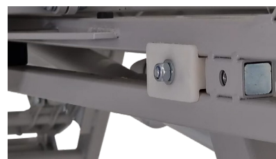
Step 6: Placing the mounts. (Right hand side when laying on the bed)
