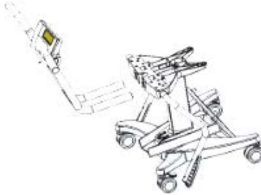
Figure 2-2. Assembling the Main Handle
